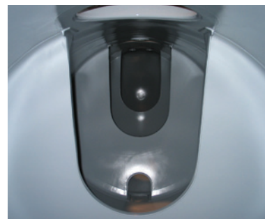
A typical baffled tank container lined with the ChemLine® coating system from Advanced Polymer Coatings.
